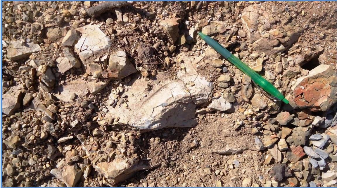
**Plate 11.** Soft crumbly mudstone all through the site and pronounced at cutting base. Suspect it Golden Valley Group, most likely Macrae mudstone. Pike et al, 1973) report that this mudstone is poorly fossiliferous and readily disintegrates on exposure to air. This lends credence to the view that the aforementioned mudstone found at the sandstone site higher up (yellow arrow) is on fact Poatina Mudstone (possibly (?) Weston Mudstone.
